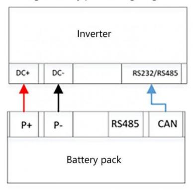
Home Energy Storage System Parallels Connection Wiring Diagram
